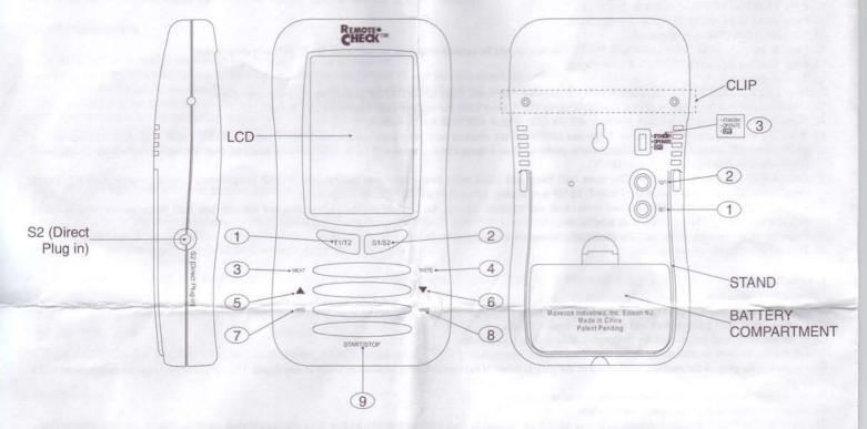
S2 (Direct Plug in) – allows you to plug 1 detachable stainless steel probe sensor directly into the receiver unit. LCD (Liquid Crystal Display) – Displays all icons, temperature and time. See LCD diagram for detailed information. CLIP – Removable clip allows you to be mobile. Clip the receiver unit to belt.
