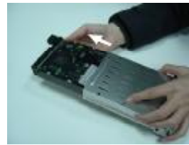
Step 5 Remove the HDD from Cartridge
