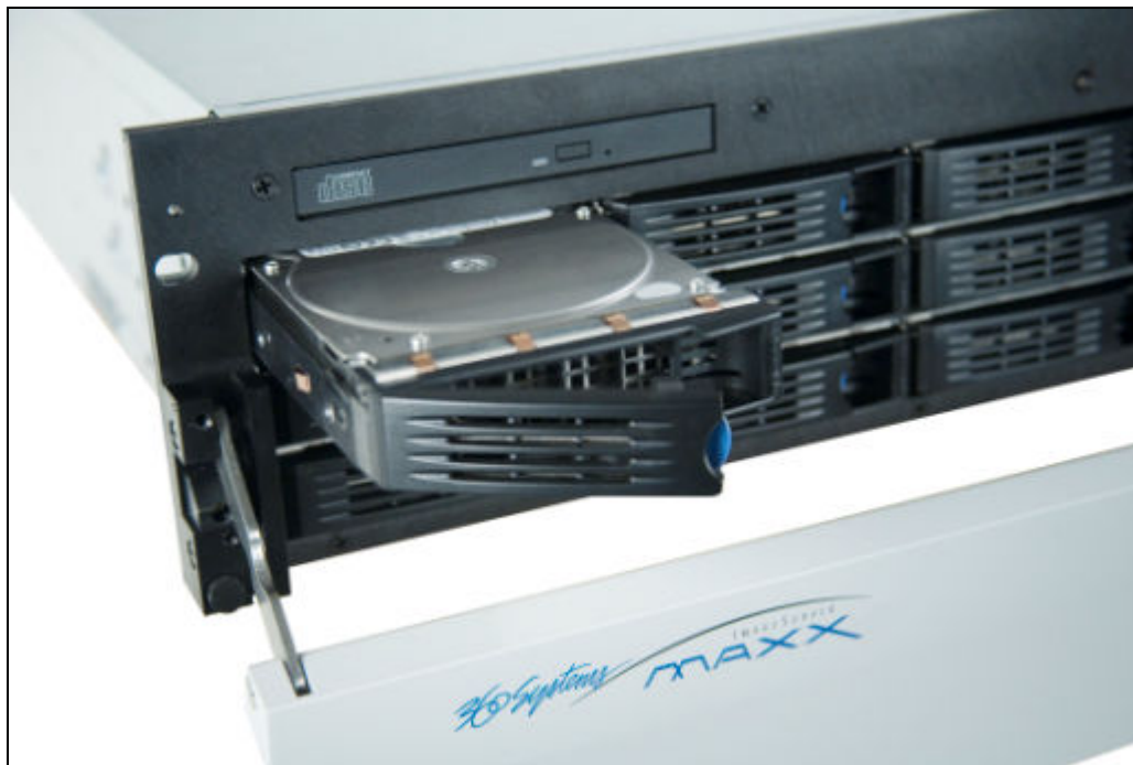
Figure 45 - Front Panel Opened – Disk Unlatched
