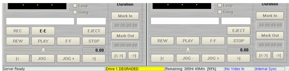
Figure 38 - GUI Drive Fault Indication
