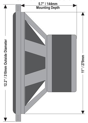
When designing an enclosure for this subwoofer, please ensure to leave atleast 2" of clearance from the back of the motor to the back of the enclosure.
