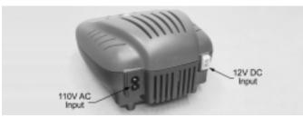
WARNING Never plug the charger into a 220V power source and never connect the charger to a 12V DC and a 110V AC power source at the same time. Use only one desired power source at a time. If connecting the charger to a 12V DC power source, make sure to attach the red alligator clip to the positive terminal and the black alligator clip to the negative terminal.
