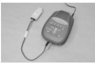
making sure that the polarity is correct (red to red and black to black), then connect your battery to the output cord.
