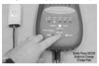
• After selecting the charge mode, select the charge rate by briefly pressing the MODE button until the desired charge rate is selected as indicated by the blinking red LED. See the table below for recommended charge rates.
