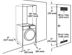
For closet installation, with a door, the minimum ventilation openings in the top and bottom of the door are required. Louvered doors with equivalent air ventilation openings are acceptable.
