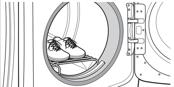
3. Place wet items on top of the drying rack. Allow space around items for air to circulate. The drying rack does not move, but the drum will rotate. Make sure items do not hang over the edges or between drying rack grille.
