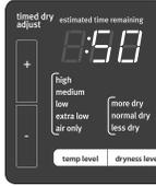
When you select a Timed Cycle, the default time appears in the display. Use the + and - buttons to increase or decrease the time in 1 minute increments. Press and hold to change the time in 5 minute increments.
