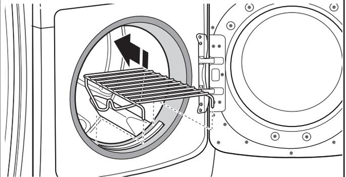
2. Align the two hooks on the front of the drying rack with the holes in the dryer door opening and press down fully into holes. Rest the rear support on the dryer back ledge.
