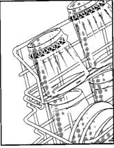
Positioning the Fold–Away tines flat in the back left corner provides convenient loading space for large, bulky items like pots and pans or mixing bowls.
