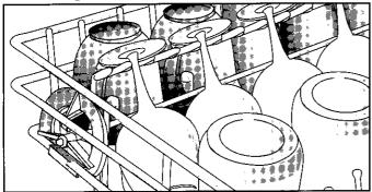
The Vari–Lock Snugger on the left (select models) can be adjusted by grasping the wire and rotating it left or right as needed. Simply move the wire to the left to snug items against the rack or to the right and rest it on top of lightweight cups or plastics. **Do not load items on top of the wire.**
