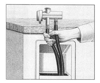
Press down on thumb release. Lift connector up on to faucet and remove pressure from thumb release to hold connector firmly in place.
