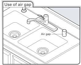
Make sure to use an air gap if the drain hose is connected to house plumbing lower than 20" (50.8 cm) above subfloor or floor.
