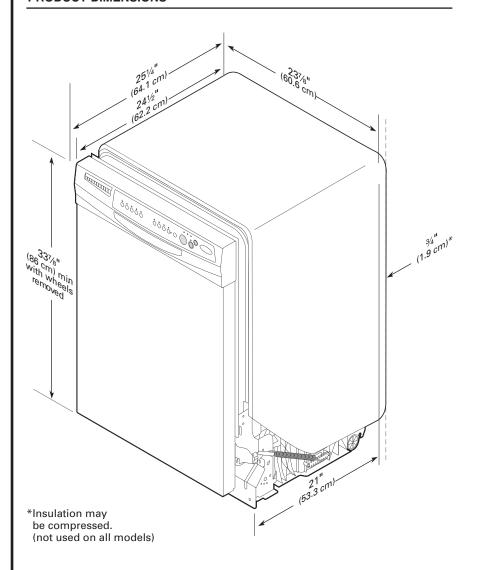
Corner locations require a 2" (5.1 cm) minimum clearance between the side of the dishwasher door and the wall or cabinet.
