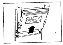
CAUTION: Hinge arms are spring mounted and will slam shut against the range if accidently hit. Never place hand or fingers between the hinges and the front oven frame. You could be injured if hinge snaps back.
