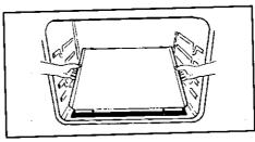
**To replace:** Fit the rear edge of oven bottom into the pin located at the center of the channel on the rear oven wall. Push toward rear of oven and lower oven bottom into place.
