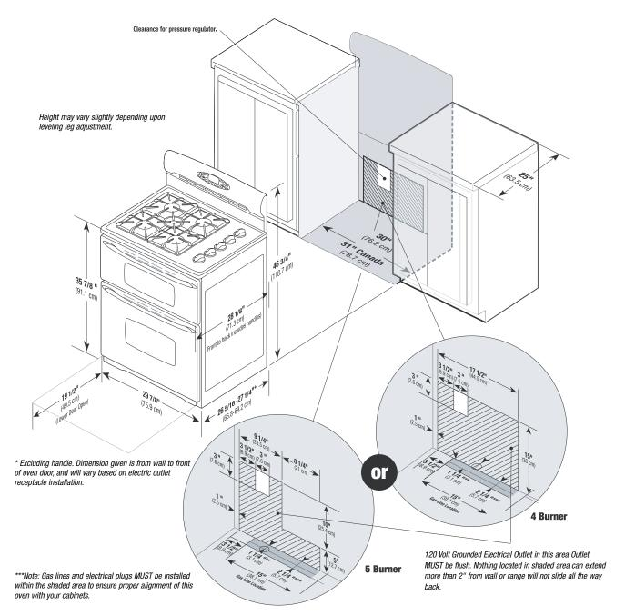
\*\*Note: Drill on centerline  $1\frac{1}{4}$ " from rear wall for gas supply line.
