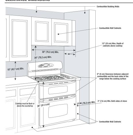
Range may be installed with zero inches clearance adjacent to (against) combustible construction at the rear and on the sides below the cooktop. For complete information in regard to the installation of wall cabinets above the range and clearances to combustible wall above the cooking top see the installation drawings. For SAFETY CONSIDERATIONS do not install a range in any combustible cabinetry which is not in accord with the installation drawings.
