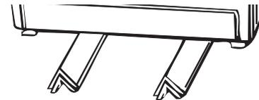
2. Use the leveling legs and nuts from the parts package. Screw nut down to within 1/2" (1.3 cm) of base.
