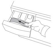
ment, press the card with your thumb and push it sideways (see illustration). The card will then bend slightly and you can easily remove it.
