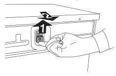
**3.** Finally, the rubber spacers should be turned over and replaced in the transport protection device holes.
