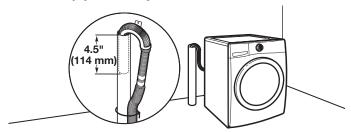
Minimum diameter for a standpipe drain: 2" (51 mm). Minimum carry-away capacity: 17 gal. (64 L) per minute. A 1/4" (6 mm) diameter to 1" (25 mm) diameter Standpipe Adapter Kit is available (Part Number 3363920). Top of standpipe must be at least 30" (762 mm) high; install no higher than 96" (2.44 m) from bottom of washer. If you have an overhead sewer and need to pump higher than 96" (2.44 m), a sump pump and associated hardware are needed. See "Alternate Parts".
