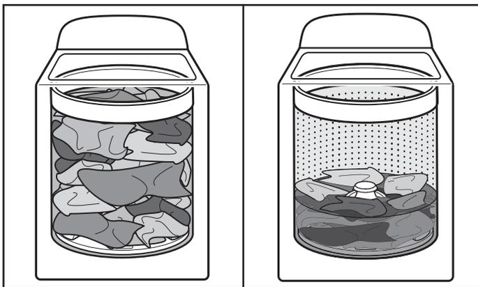
As the washer dampens and moves the load, the level of the garments will settle in the basket. This is normal, and does not indicate that more garments should be added.
