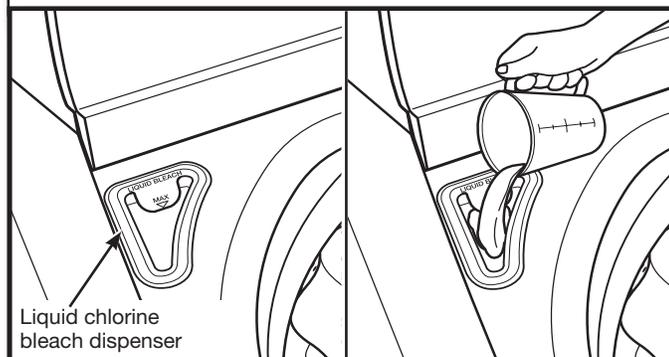
Do not overfill, dilute, or use more than 3/4 cup (180 mL). Do not use color-safe bleach or Oxi products in the same cycle with liquid chlorine bleach.
