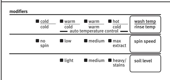
Once you select a cycle, the default settings for that cycle will be lit. Press the Modifier buttons to change the Soil Level, Spin Speed, and Wash/Rinse Temperature, if desired. Not all settings are available with all cycles.
