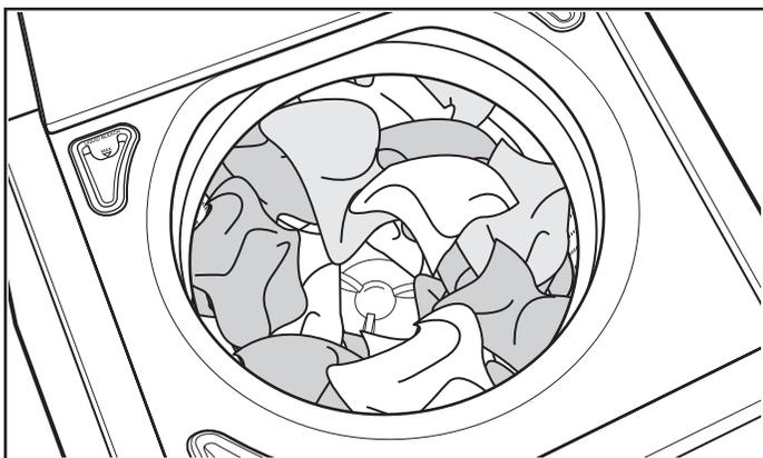
Load garments in loose heaps evenly around the washplate. Do not load garments directly over the center of the washplate; when loaded, the center of the washplate should be visible.
