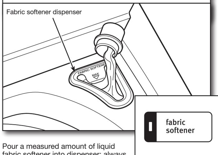
Pour a measured amount of liquid fabric softener into dispenser; always follow manufacturer's directions for correct amount of fabric softener based on your load size. Then select Fabric Softener option.
