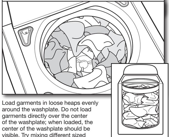
Load garments in loose heaps evenly around the washplate. Do not load garments directly over the center of the washplate; when loaded, the center of the washplate should be visible. Try mixing different sized garments to reduce tangling.
