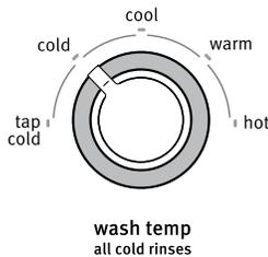
Once you select a cycle, select the desired wash temperature by turning the Wash Temperature knob to the appropriate setting based on your load. All rinses are cold.
