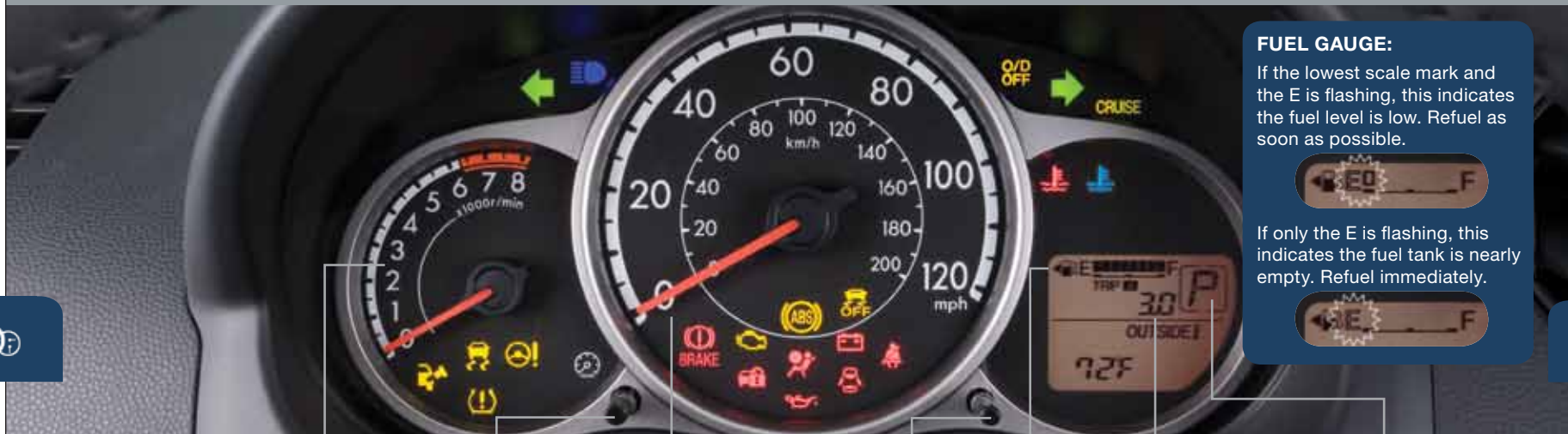
TACHOMETER DASHBOARD ILLUMINATION 1 SPEEDOMETER TRIP METER SELECTOR 2 FUEL GAUGE ODOMETER/TRIP METER SHIFT LEVER POSITION INDICATOR (AUTOMATIC TRANSMISSION ONLY)
