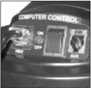
Fig. 10: Connect Autostar to the HBX port.
