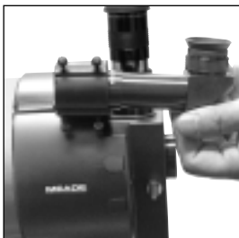
Fig. 8: Attach the viewfinder to the viewfinder bracket.
