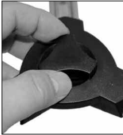
Fig. 6b: ...turn the locking ring to secure the tripod legs.
