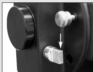
Fig. 31a: Flip mirror control in the “up” position.
