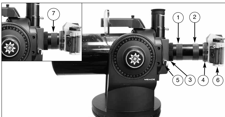
Fig. 30: Example of photography through the ETX using the #64 T-Adapter: (1) Short section of #64 T-Adapter; (2) Extension section of #64 T-Adapter; (3) Knurled attachment ring; (4) T-mount; (5) Flip-mirror control in “up” position; (6) 35mm camera body; (7) Format 1.
