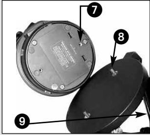
Fig. 11: High latitude leg mounting hole and corresponding attachment knob.
