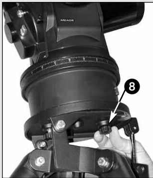
Fig. 12: Attach telescope to tripod.
