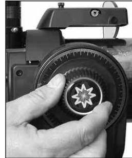
Fig. 16: Tighten vertical lock.
