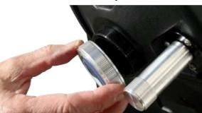
Attach spreader bar and secure with washer and knob.
