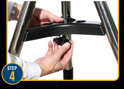
• Center telescope base onto tripod head and fasten three screw knobs to a firm feel.
