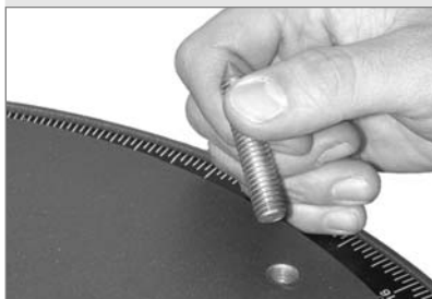
Fig. 51: Remove the pointed bolts from the drive base.
