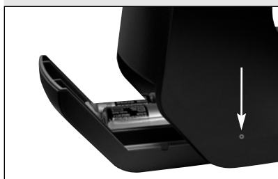
Fig. 59c: Location of one of the battery compartment screws. The other is located on the opposite end of the horizontal beam of the fork arms near the other battery compartment (older models).
