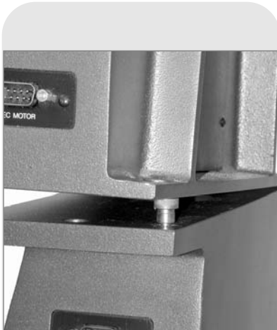
Fig. 56: Position the holes over the shoulder bolts. When they are in place, slide the OTA back so that the shoulder bolts lock into the slots.
