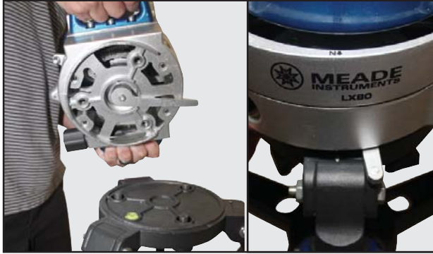
Fig 15: Place mount base on tripod. Point the “N” on the front of the mount to True North.
