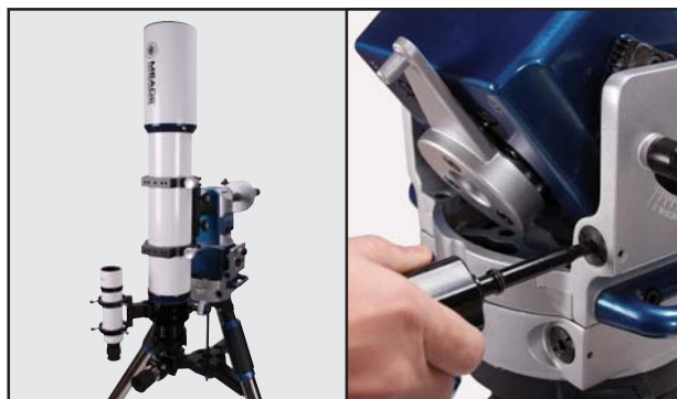
Fig 35: Tilt the mount head using hex head tool
