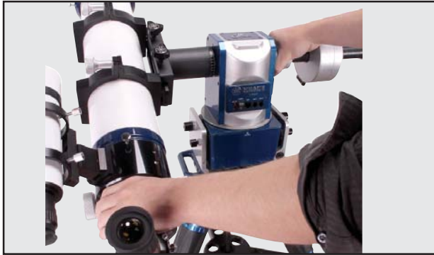
Fig 25: While maintaining hold of OTA, loosen the DEC lock
