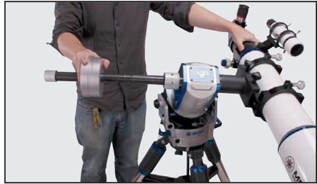
Fig 31: Adjust counterweight to achieve balance
