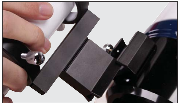
Fig 21: Slide in finderscope and secure
