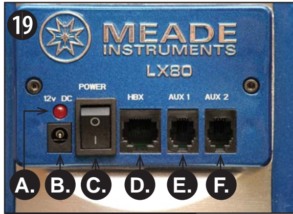
Figure 3: LX80 Control Panel - Detail
