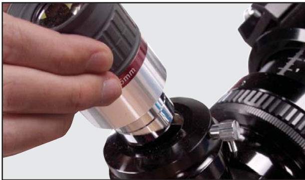
Fig 23: Insert eyepiece into diagonal
