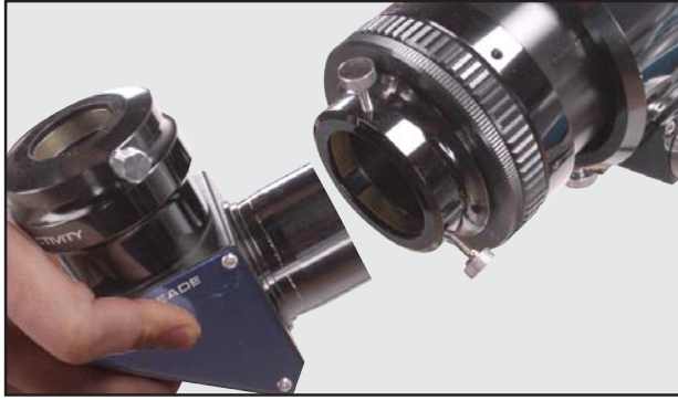
Fig 22: Secure diagonal into holder
