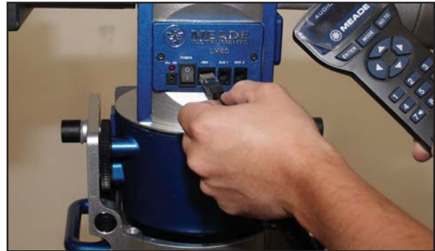
Fig 24: Plug AudioStar into HBX connector
