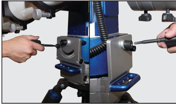
Fig 28: Loosen RA lock – right and left sides
