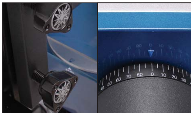
Fig 34: Align “EQ” with “AZ/EQ” mark. Set OTA at “0” mark
