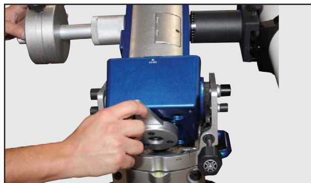
Fig 30: Disengage the RA lock
