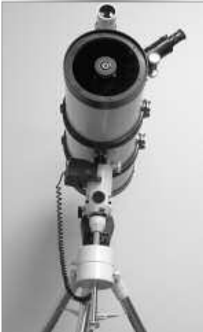
Fig. 16a: The polar home position, side view. Inset: Line up triangles on the mount.
