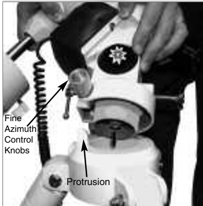
Fig. 4: Attach the mount to the tripod.
