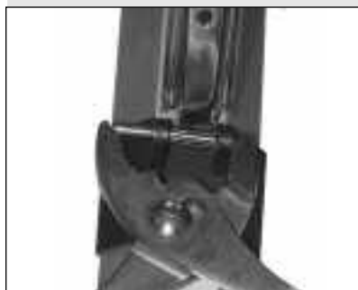
Fig. 7: Attach pin to tripod leg bracket with a large pliers (Style 2).
