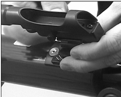
Fig. 10a: Attach red dot viewfinder to the optical tube.
