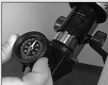
Fig. 12: Remove the eyepiece and slide in the compass/ bubble level.
