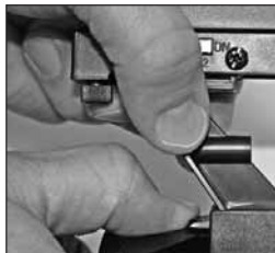
Fig. 8b: Press down on the quick release tab to detach the viewfinder from the bracket.
