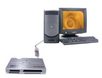
Connect your card reader to your PC (note: be sure that the card reader driver is installed) and insert the Compact FLASH card (we recommend 128 MB minimum) into the reader. To program your multimedia content on to the media card, open the file manager and copy the files to the card reader drive.
