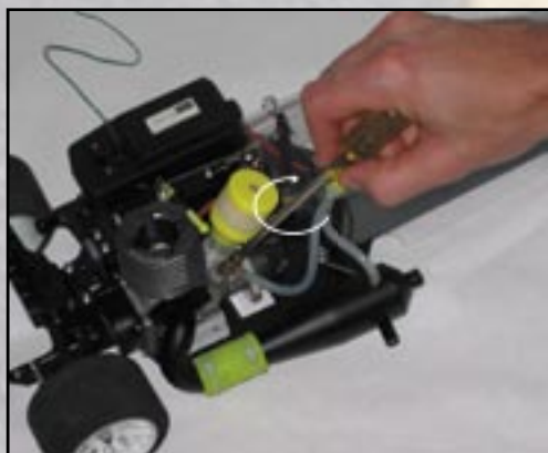
Figure 9 - Closing the high speed valve
