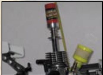
Figure 13- Glow plug ignitor
