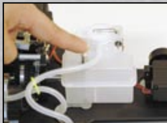
Figure 12- Priming the engine
