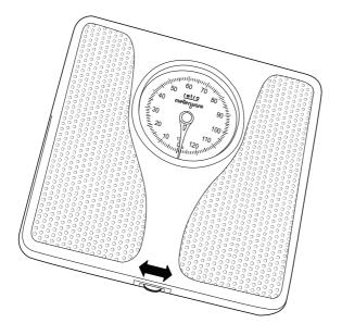
Adjust the calibrating dial left or right to set the scale to zero (0).
