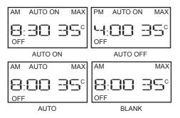
The booking timing mode setting can be circulated as above sequence and the yellow timing pilot light will be on during the heater operating in auto mode.
