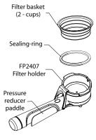
pressure reducer firmly (hold for 5 seconds) when removing the filter holder, so that the pressure remaining in the filter will be release and the filter can be removed safely.
