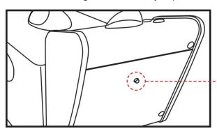
Reset button shown at the rear of the heating element assembly.
