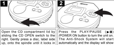
right. Gently press a disc, label side up, onto the spindle until it locks in place. Close the CD compartment lid. Insert headphones into the PHONES jack.
