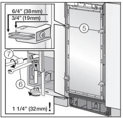
The installation aids (5) have been designed for the following total thickness of custom doors:
