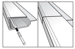
Take the peg from the "side-by-side merging kit" and insert it halfway into the filler strip rail on the left-side appliance.
