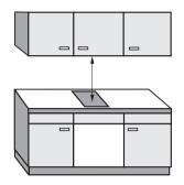
The minimum safety distance given by the hood manufacturer must be maintained between the cooktop and the hood above it. See the installation instructions of the hood for these safety measurements.
