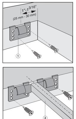
Place the supplied spring clips ① and the support bars ② at the marked positions as shown above, by laying them on the upper edge of the cut-out and then securing them with the <sup>1</sup>/<sub>8</sub>" x 1" (3.5 x 25 mm) screws (supplied).
