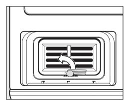
■ Turn the lever on the condenser unit to the vertical position so that the hook on the lever is no longer in the groove at the bottom of the condenser unit housing.
