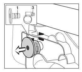
Remove the following from the back of the dryer at the top: Adapter 1 and hose clip 3 behind it.
