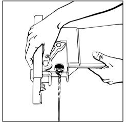
Pull forward the cap of the spout as indicated by the arrow and hold open while emptying the container.
