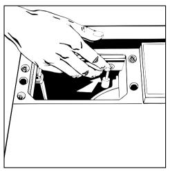
Close the water inlet port above the condensed water container with the bottom part of the rubber plug. The plug must face towards the interior of the machine so that the condensed water container can easily be inserted. Connection to wash basin drain outlet
