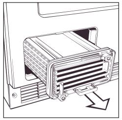
Pull out the heat exchanger
