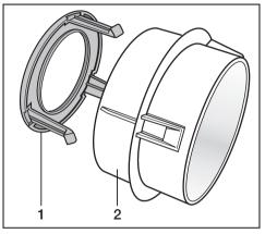
The adapter, **1**, is inserted into the connector, **2**.
