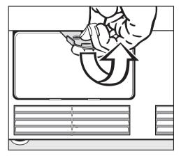
Open the access panel, located on the lower left corner of the machine, using the yellow tool supplied with the machine.
