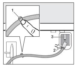
Unclip the drain hose from the clamps 1 and 2, and pull it off the holder, 3.
