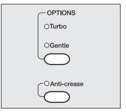
A drying option can be selected or deselected with each press of the button. 4. Select the dryness level
