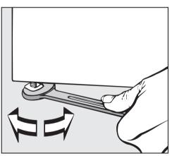
The machine can be leveled by turning the legs clockwise or counterclockwise as necessary.
