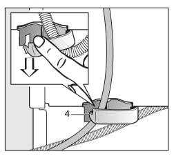
■ The lower clamps, **4**, can be opened to install the drain hose or to feed the power cable through.
