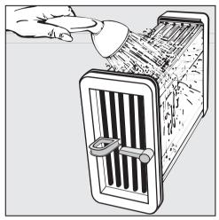
Check the condenser for visible soiling. Continue rinsing until the condenser until clean.
