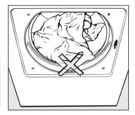
When closing the door make sure items of laundry cannot be trapped by the door, as this will cause damage to the laundry.
