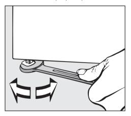
■ The screw feet can be adjusted to compensate for any unevenness in the floor.
