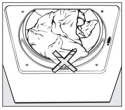
Check the laundry is right inside the drum so that it cannot get trapped or damaged when the door is shut.
