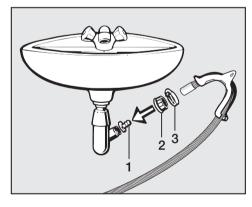
Fit adapter 1 to the sink drain outlet using nut 2. If this nut has a flat disc in it you should take the disc out first. Important: if this nut has a washer or seal in it this must not be removed!
