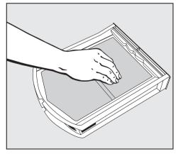
Use your fingers to remove the fluff from the surface of the filter.
