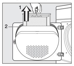
Open the door and pull the fluff filter(1) out of the door as illustrated.
