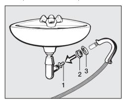
■ Fit adapter 1 to the sink drain outlet using nut 2.
