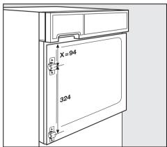
Mark the two hinge holes and the four smaller holes as shown in the diagram.
