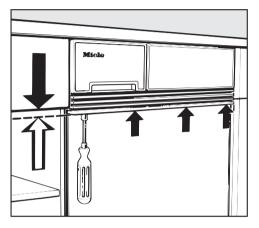
Using a socket spanner, turn clockwise or anti-clockwise until the required height is reached.
