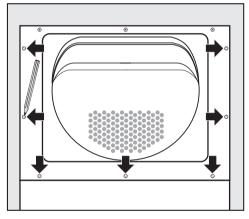
Mark the fixing points on the back of the front panel through the holes in the machine door plate (see arrows in the illustration).
