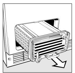
■ Pull out the heat exchanger
