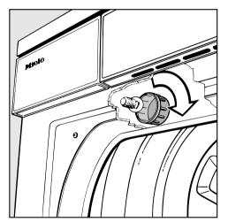
■ Use a 19 mm spanner to unscrew the plastic cover inside the drum above the door.
