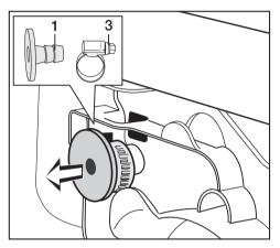
Remove the accessories from the top of the rear side of the dryer: Adapter 1 and the hose clip 3 behind it.
