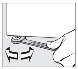
Compensate for floor irregularities by turning the threaded feet in or out.
