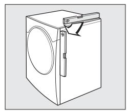
To ensure trouble-free operation, the dryer must be level.
