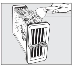
Rinse the unit from the longitudinal side with a stream of water – as shown in the top illustration.
