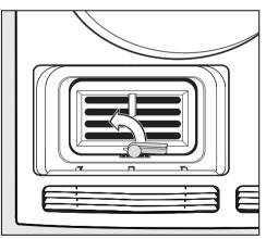
Rotate the locking lever on the condenser upward (the locking lever hook disengages from the groove in the base).
