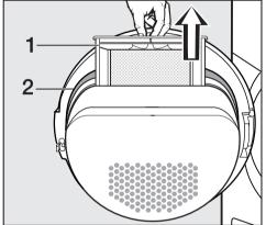
Pull the door lint filter (1) out of the door casing.
