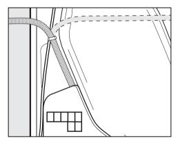
Guide the hose to the right or left side of the dryer, as necessary.
