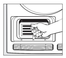
Pull the condenser by its <u>handle</u> out of its housing.
