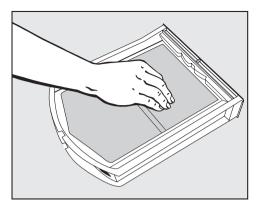
■ Use your fingers or a vacuum cleaner to remove the fluff from the surface of the filter.
