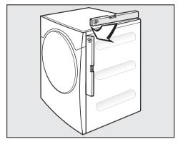
The dryer must be perfectly level to ensure safe and proper operation.
