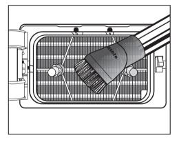
Remove any visible soiling carefully with a vacuum cleaner using a dusting brush or a narrow crevice nozzle.
