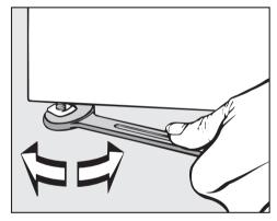
■ The screw feet can be adjusted to compensate for any unevenness in the floor.
