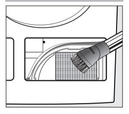
Vacuum up any soiling carefully using a vacuum cleaner dusting brush or small crevice nozzle.
