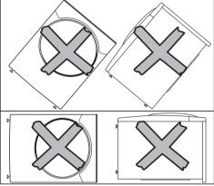
If the tumble dryer has not been transported as described, then it must be left to stand for at least 1 hour <u>before</u> it is connected to the electricity supply. Otherwise the heat pump can be damaged.
