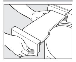
Pull out the condensed water container. ■ To prevent water running out, hold it at the front and towards the back and keep it in a horizontal position when carrying it.
