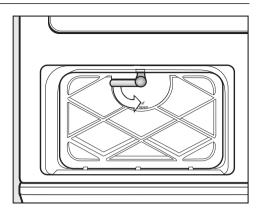
Turn the condenser door lock down and remove the door up and out.
